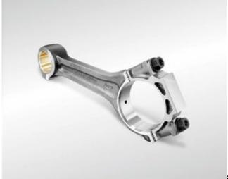
converts the linear up and down movement of the piston into the circular motion of the crankshaft and is therefore subject to tension, compression, bending and buckling.
