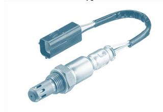
The engine control unit uses this voltage signal to determine the current mixture composition. With binary lambda sensors, the sensor signal switches back and forth between two values. Depending on the composition, the quantity of fuel injected is reduced (rich mixture) or increased (lean mixture).
